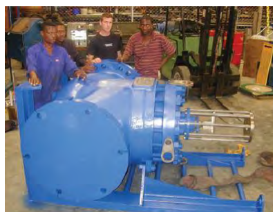
Twin Pump Test Valve
